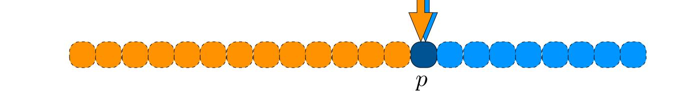
$(i, A[1, \ldots, n])$ RandomizedSelect PICK RANDOM PARTITION ELEMENT PARTITION LIST ABOUT THIS ONE IF PIVOT IS POSITION i, RETURN PIVOT ELSE IF PIVOT IS IN POSITION > i select  $(i, A[1, \dots, p-1])$ ELSE SELECT ((i - p - 1), A[p + 1, ..., n])
