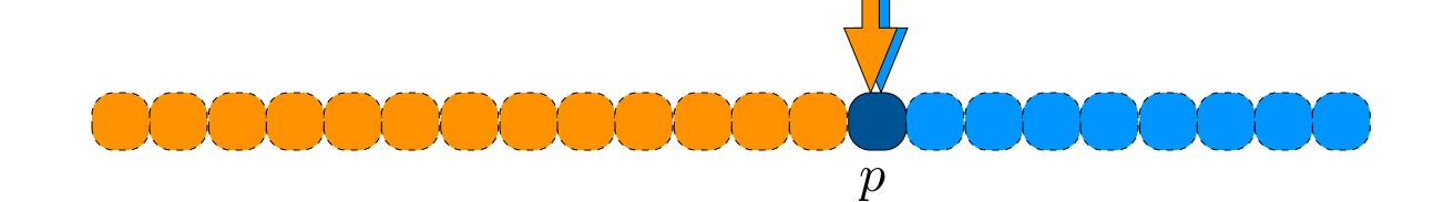
SELECT  $(i, A[1, \ldots, n])$ **PICK FIRST ELEMENT** PARTITION LIST ABOUT THIS ONE IF PIVOT IS POSITION i, RETURN PIVOT ELSE IF PIVOT IS IN POSITION > i select  $(i, A[1, \dots, p-1])$ Else select ((i - p - 1), A[p + 1, ..., n])
