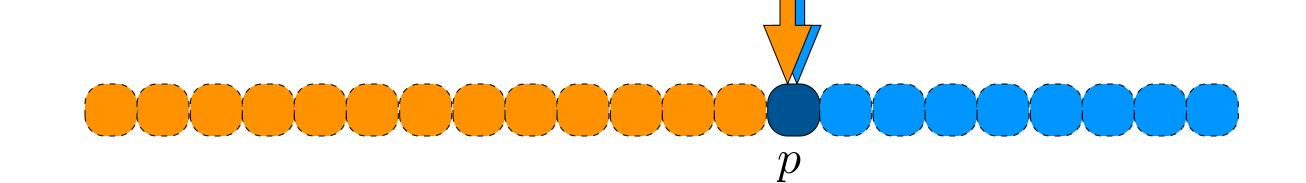
**SELECT** (i, A[1, ..., n])**PICK FIRST ELEMENT** PIVOT = PARTITION  $(A[1,\ldots,n])$ IF PIVOT IS POSITION i, return pivot ELSE IF PIVOT IS IN POSITION > i select  $(i, A[1, \dots, p-1])$ ELSE SELECT ((i - p - 1), A[p + 1, ..., n])
