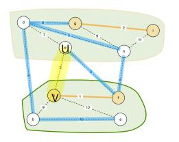
As an example, the set A is in orange. The edge e is yellow and T is blue. We will construct a T' which includes A+e.
