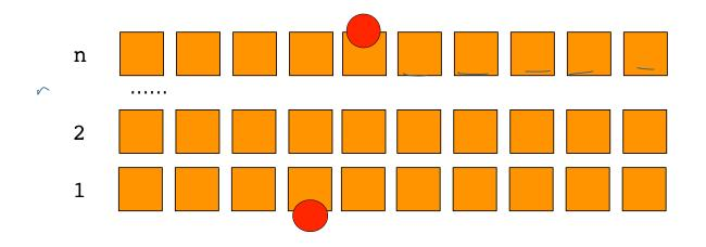
RUNNING TIME start at bottom of picture. initialize  $S_1(i) = e(1, i)$ for i=2, n use formula to compute  $S_{i+1}(\cdot)$  $S_i(j) = e(i,j) + \min \begin{cases} S_{i-1}(j-1) \\ S_{i-1}(j) \\ S_{i-1}(j+1) \end{cases}$
