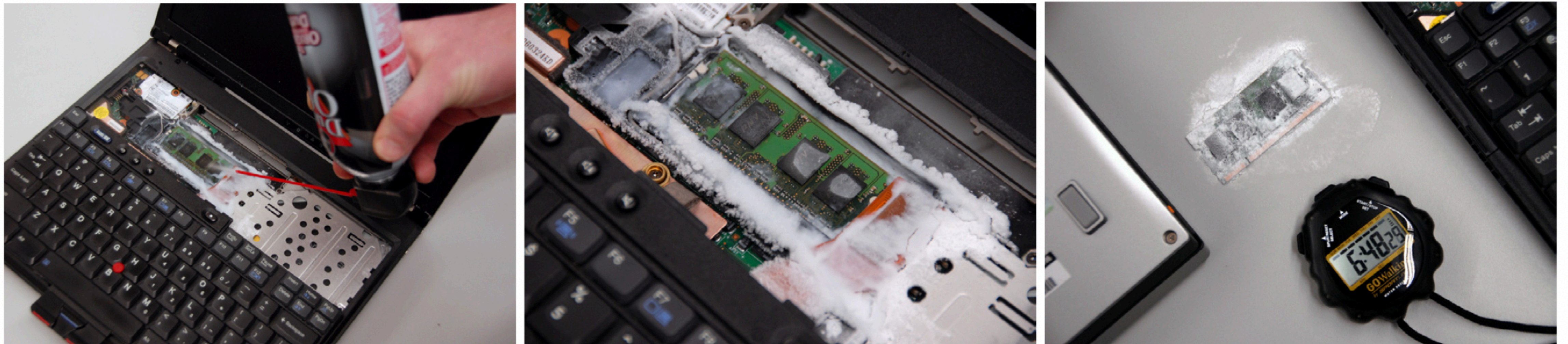
Figure 5: Before powering off the computer, we spray an upside-down canister of multipurpose duster directly onto the memory chips, cooling them to -50^{\circ}\text{C} . At this temperature, the data will persist for several minutes after power loss with minimal error, even if we remove the DIMM from the computer.
