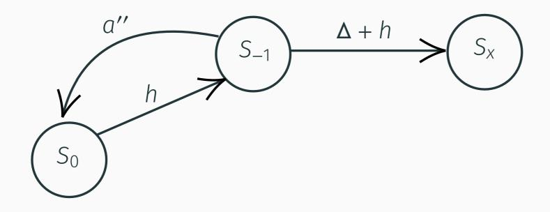
State  $S_{-1}$ : honest chain ahead by one block.  $S_x$ : attack has failed
